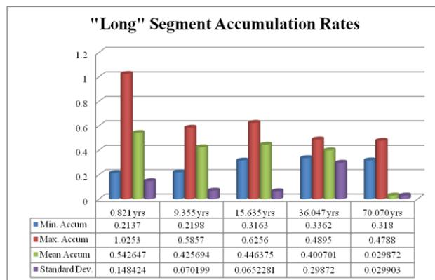
**Figure 10:** Depicting the shallowest “long” digitized layer (0.311 m) and the deepest digitized layer (52.24 m), the chart also included the age of the layer, minimum accumulation rate, maximum accumulation rate, variation in mean, and standard deviation for each digitized firn layer.
