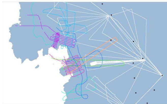
**Figure 12:** An image in ArcMap<sup>®</sup> of the 2009 Operation IceBridge flights (represented by the colored lines), the ITASE core sites (represented by the black dots), and the flight path of the CreSIS developed accumulation radar used by Ms. Brooke Medley to derive accumulation rates of Antarctica (2009-2010).
