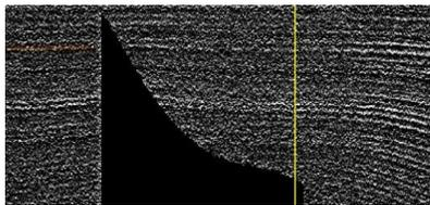
**Figure 4:** Potentially due to radar operation issues, there are information gaps. These information gaps can omit temporal and geospatial data ranging from shallow layers to deeper layers, as well as spanning meters to several kilometers of data when exported to ArcMap® and geospatially (latitude and longitude) referenced.
