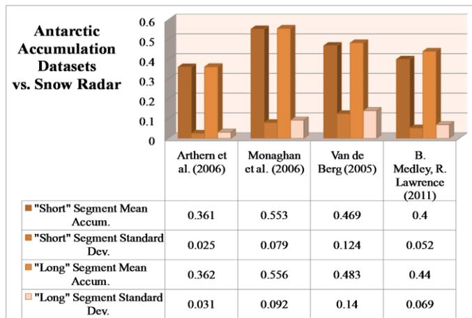
**Figure 11:** Continent wide datasets (specifically measurements of the variation in mean and standard deviations for the "short" and "long" segments) from Arthern et. al (2006), Monaghan et. al (2006), and van de Berg (2005) were compared to the derived Thwaites Glacier dataset from Ms. Brooke Medley and Mr. Ryan Lawrence.
