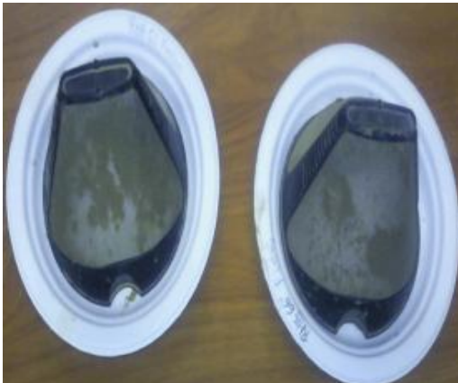
Figure 5. Shows two filters containing the floating material extracted.
