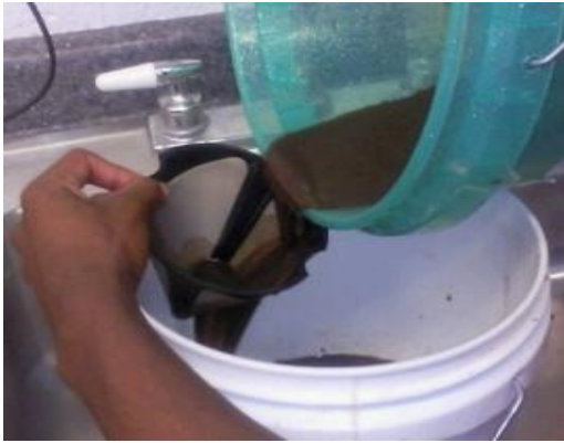
Figure 4. Shows the slurry being filtered through a 20-micron mesh filter.
