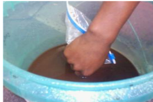
Figure 6. Shows the magnet being slowly moved around the slurry.
