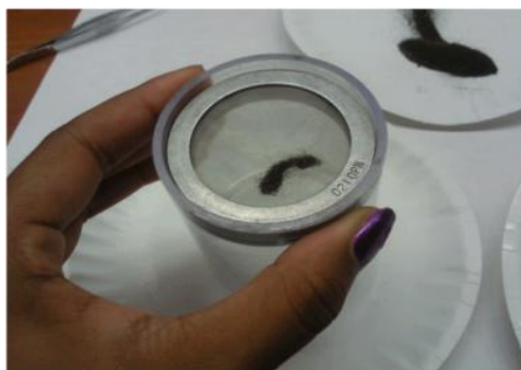
Figure 8. Size sorting of magnetic grains.
