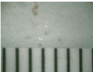
Nano-diamonds presumably created in an environment of intense heat and pressure (Sample 1 SMCBMD diamond extract 2scale shows 3 such nano-diamonds with a millimeter scale)
