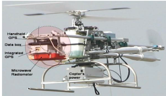
Figure 2. Autonomous drone model--a performance UAV for microwaves/infrared classroom/lab projects [11].
