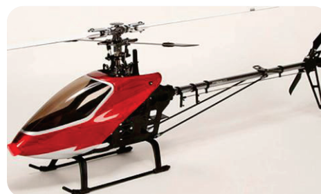
Figure 1. HK-500GT model data collector, a performance UAV customized for classroom/Labs
