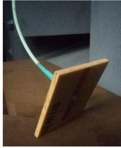
Figure 7: Microstrip antenna setup in anechoic chamber
