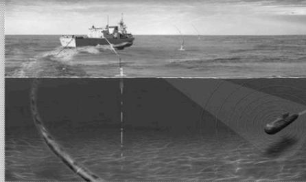
Remote sensors fall into 2 categories. Active and passive. Active sensors provide their own source of illumination. Examples are the radar which is used for speed detection, lidar for ground detection and sonar to find ships and submarines.
