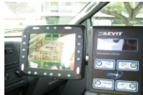
Drive-by-wire system actuates steering, throttle, and brakes
